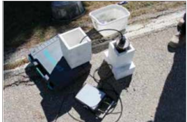
Fig. 2 UPV test set up for a sample in wooden frame 1
