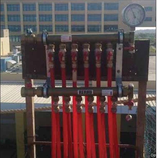
*Fig 3 Piezometer connected to network of pipes*
